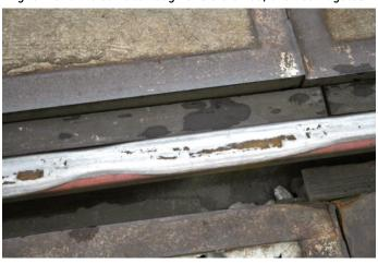
The wear on the railhead is particularly acute on curves, and rail grinding trains might need multiple passes to get the railhead ground to just the right profile given the degree of curve, train speeds, and train weight. This calls for careful analysis of the rail line, and careful control over the grinding mechanisms. The host railroad and the rail grinding experts arrive at detailed grinding plans before work commences.
