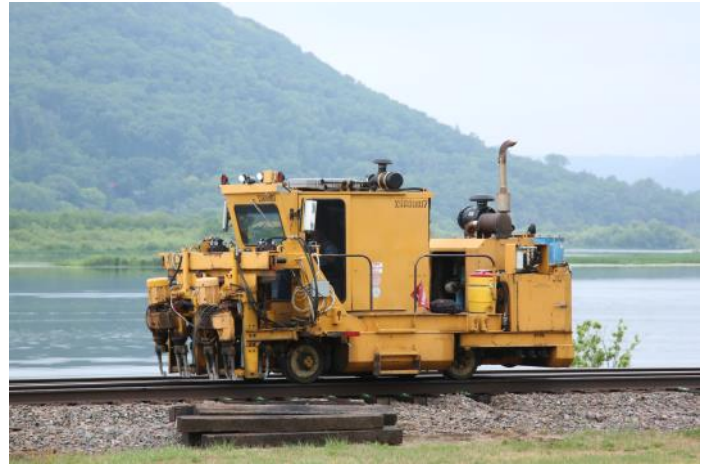
This tamper squeezes ballast under the ties to provide a strong and stable foundation for the track structure. This machine did not appear to be working, at least not in front of our reviewing stand.
