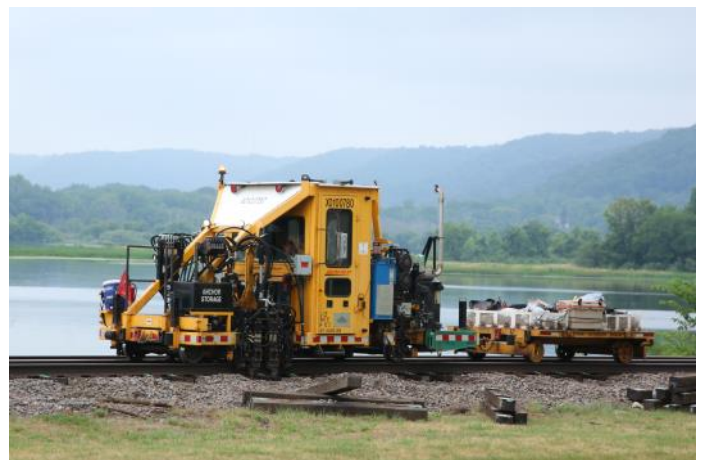
The Racine DAA (Dual Anchor Adjuster) pushes the rail anchors tight up against the new ties. This machine rides on a chassis similar to the DASP seen earlier. The toolheads are oriented to squeeze the anchors, not spread them.
