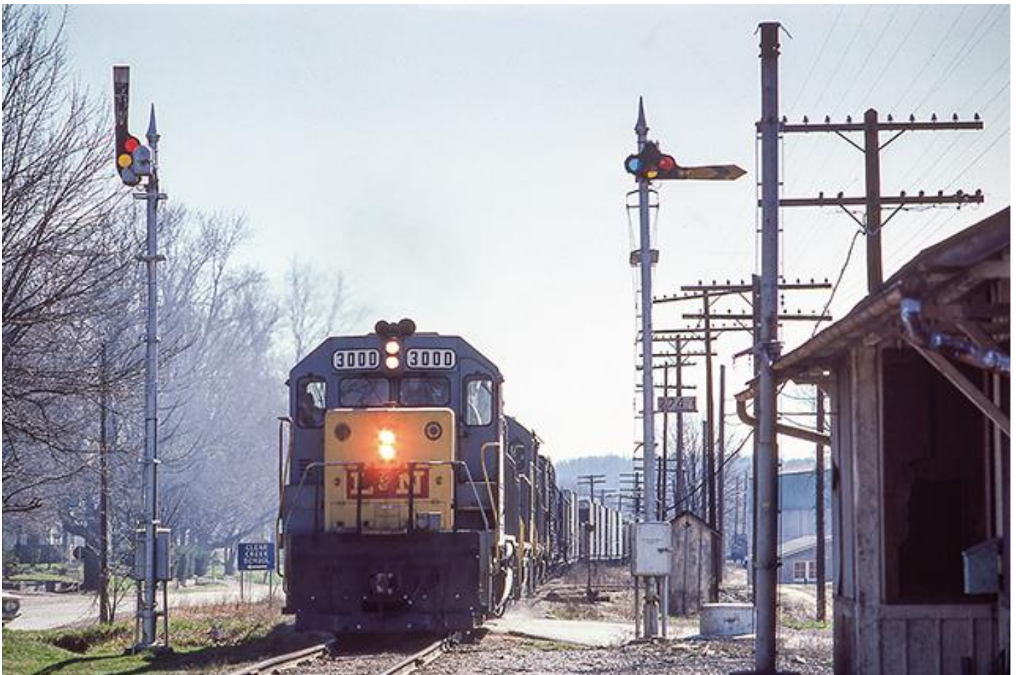
Louisville & Nashville number 3000, the GP40 class unit, leads a train north on the former Monon at Clear Creek, Indiana. The locomotive was built for the road in October of 1966. This is late winter or early spring, which provides back-light that illuminates the colored lenses of the semaphores located here by the small frame depot, which is out-of-service by this time. The train will soon be at McDoel yard just south of Bloomington. Photo by Richard Koenig; March 6, 1976
